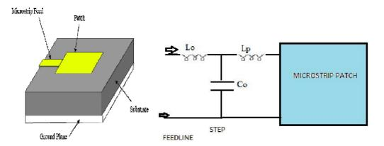
Fig. 3.1 Microstrip line feed and its circuit diagram
