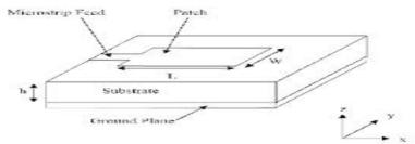
Fig.1 Micro strip Patch antenna
