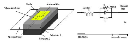
Fig.3.3 Aperture-coupled feed and its Circuit diagram
