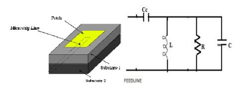
Fig.3.4 Proximity-coupled Feed and its circuit diagram
