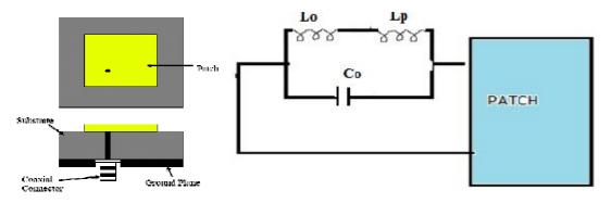
Fig.3.2.Probe fed micro strip patch antenna and its circuit diagram
